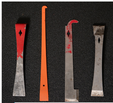
Figure 1. Standard, J-hook, and other hive tools
